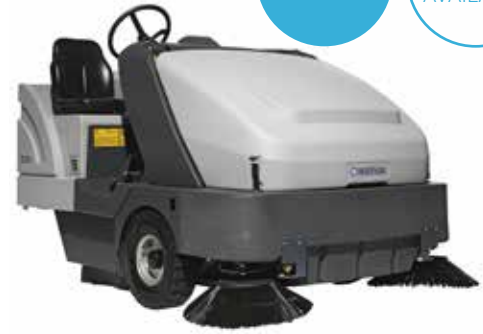
Left and right side brooms are standard spec on Maxi models.
